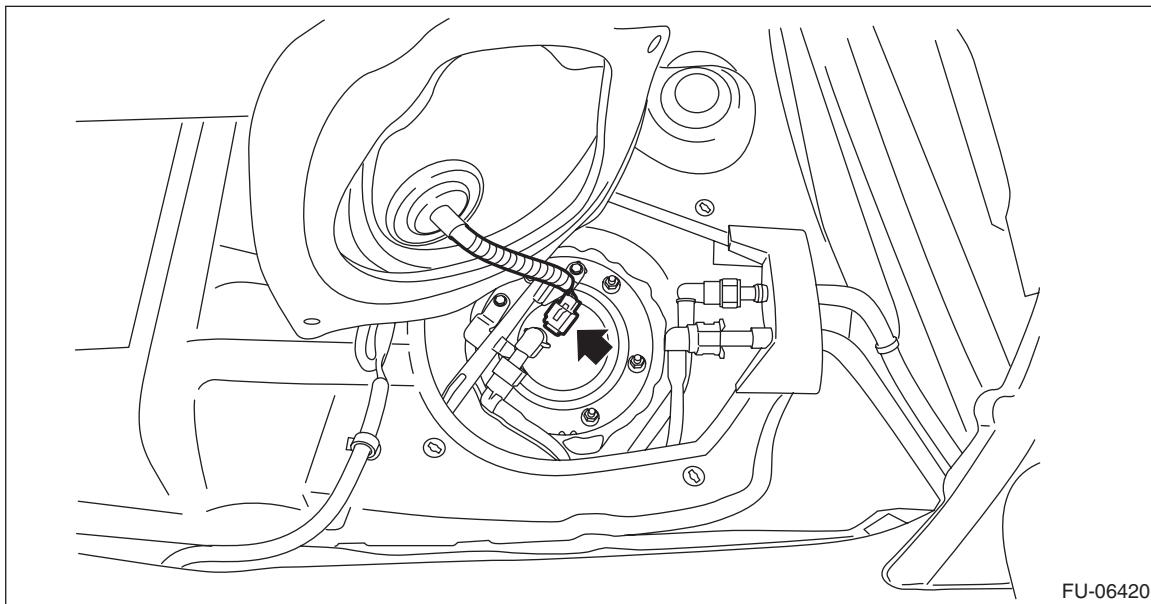
7) Disconnect the quick connector of the jet pump tube.
