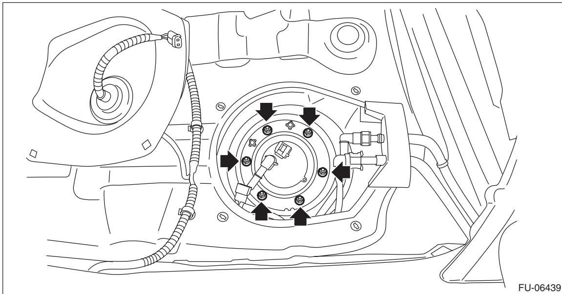
10) Remove the fuel sub level sensor from the fuel tank.
